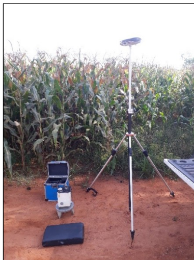
Figure 3 - Gravimetric survey accompanied by GNSS measurement.
