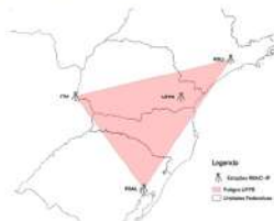
Figure 2: Possible geometry for generation and application of atmospheric corrections
