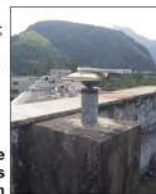
Figure 4: Smartphone collecting observations at the geodetic station
