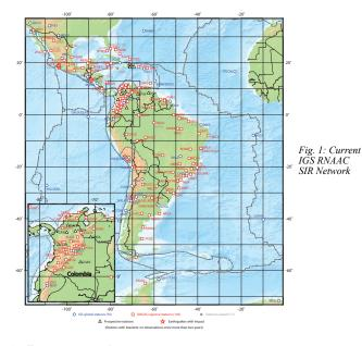
**2. Reprocessing:** The IGS RNAAC SIR reprocessed 168 weeks between 2002 to 2007 (GPS weeks 1147 to 1450). The reprocessing of the missing weeks of 2003/2004, and of the second half of 2005 is in progress. All weeks are computed with the Bernese Processing Engine (BPE) version 5.0 using absolute phase centre corrections instead of relative. The reference frame is IGS05, with 18 IGS05 fiducial stations in the RNAAC SIR region (see Fig. 2a).
