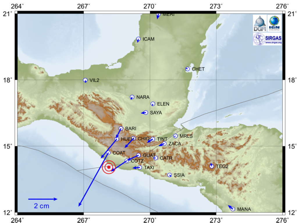
Horizontal displacements of the SIRGAS Reference Frame estimated after the earthquake 7.4M of 2012-11-07 in Guatemala
