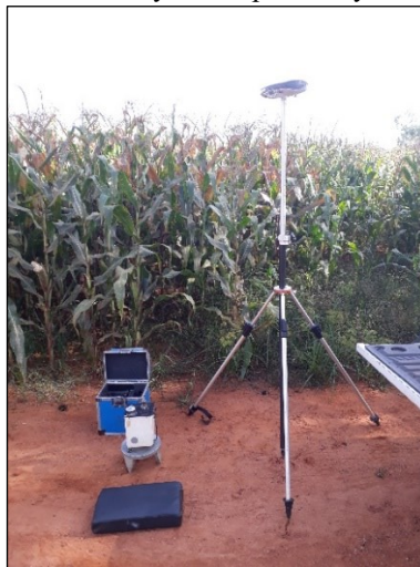
Figure 3 - Gravimetric survey accompanied by GNSS measurement.
