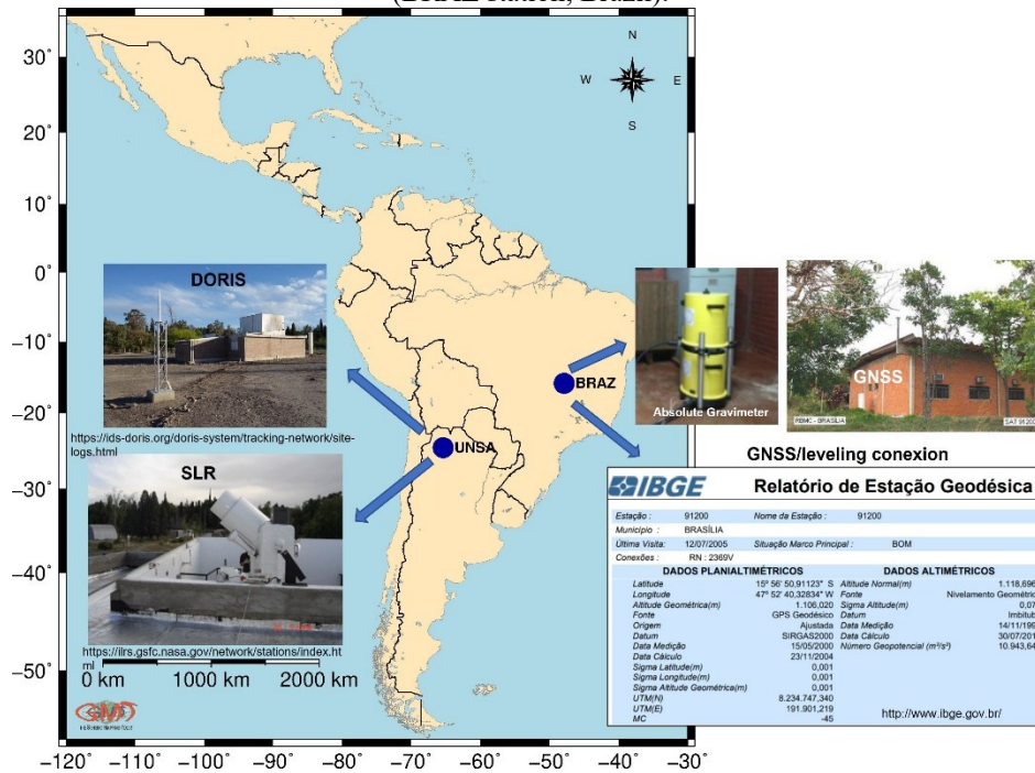
Figure 1 - Example of a co-located IHRF station (UNSA station, Argentina) and an IHRF station with absolute gravity measurement and connection to the local Vertical Datum - GNSS / leveling (BRAZ station, Brazil).
