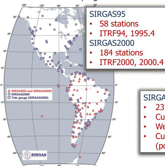
Now: Realization by means of a continuously operating GNSS network (SIRGAS-CON)
