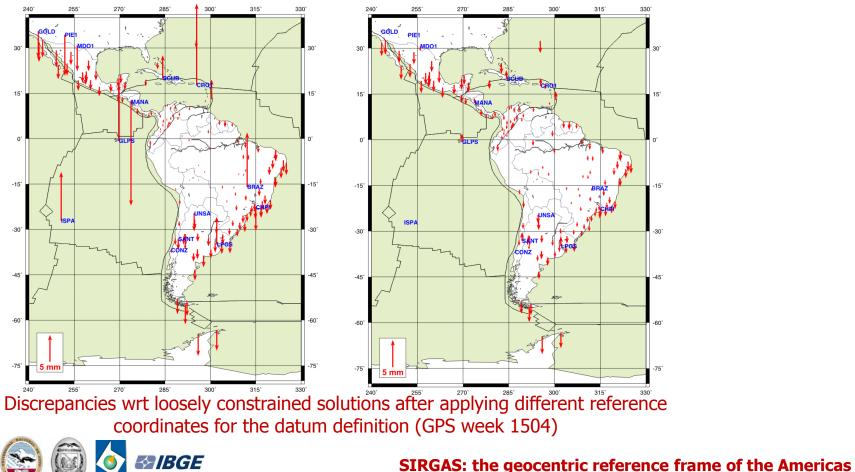
Now: Reference positions are computed by aligning the weekly solutions of the SIRGAS frame to the same frame in which the GNSS orbits are computed, i.e. the IGS weekly solutions.
