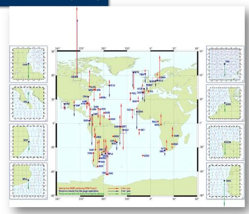
Combined analysis of tidal records, satellite altimetry and GNSS positioning in order to unify the local vertical reference systems
