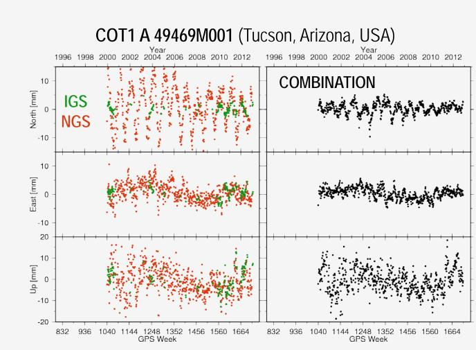
Figure 5: Residual position time series with respect to cumulative solution of individual weekly regional solutions (left) and weekly combined solution (right).
