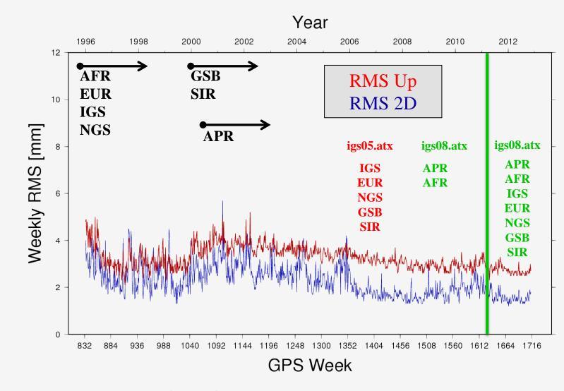
Figure 2: RMS [in mm] of the weekly combinations as a function of time (Up in red and 2D horizontal in blue)
