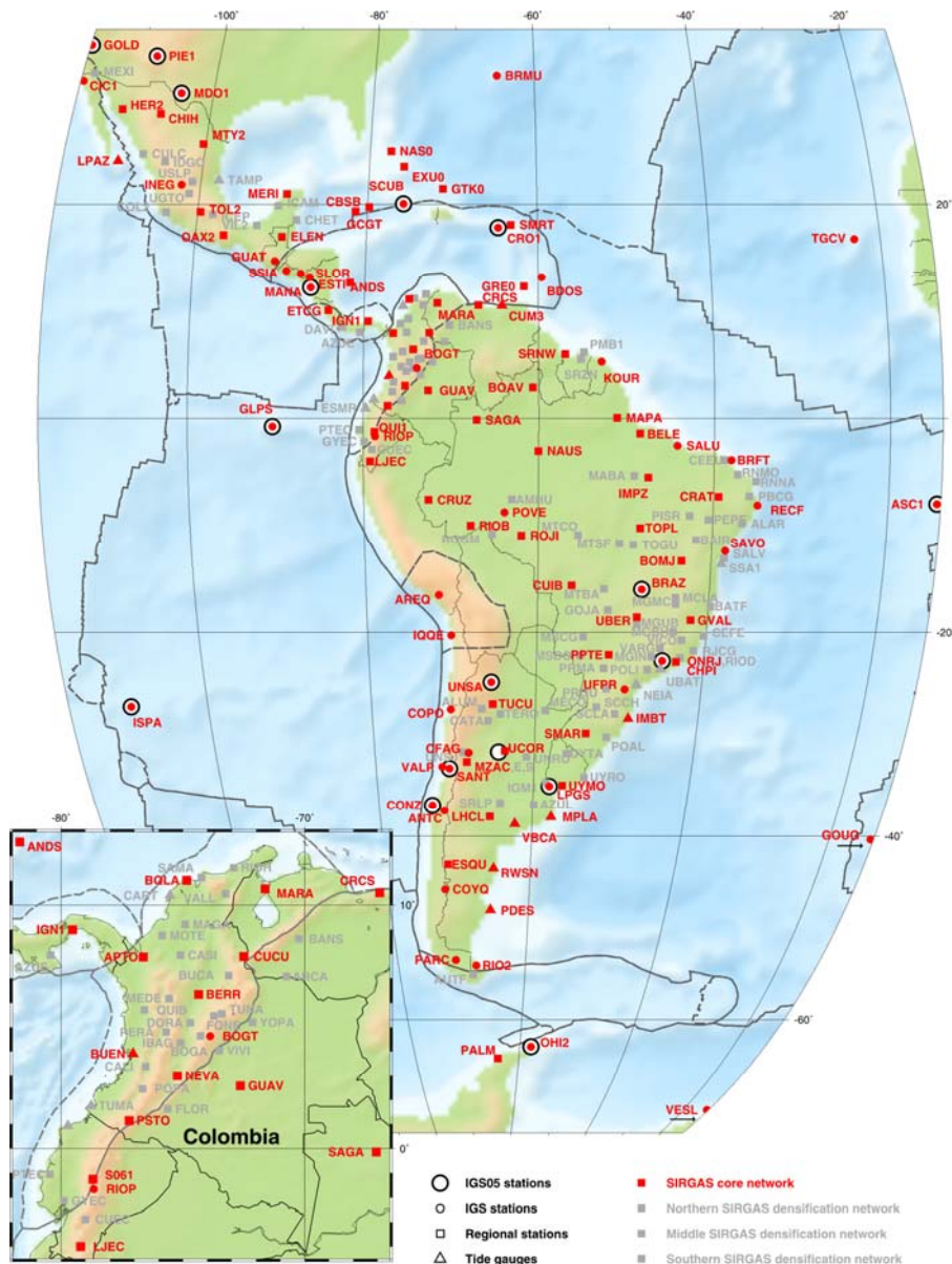
Figure 1. SIRGAS-CON-C core network: DGFI processes routinely this network and provides loosely constrained weekly solutions to be combined with the SIRGAS-CON-D densification sub-networks.
