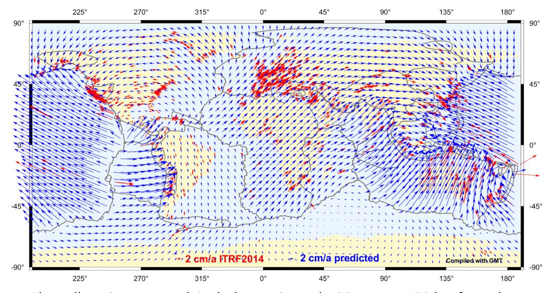
The collocation approach includes station velocities up to 500 km from the grid point to be predicted. If a sufficient number of station velocities (> 3) is not available, the used plate model (APKIM2014) is considered.
