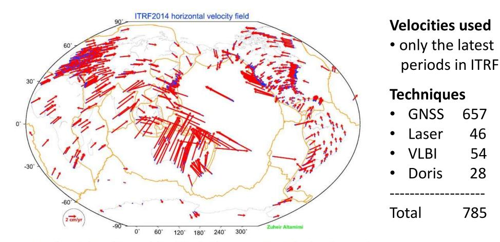
**Figure 11.** ITRF2014 horizontal site velocities with formal error less than 0.2 mm/yr. Major plate boundaries are shown according to *Bird* [2003].
