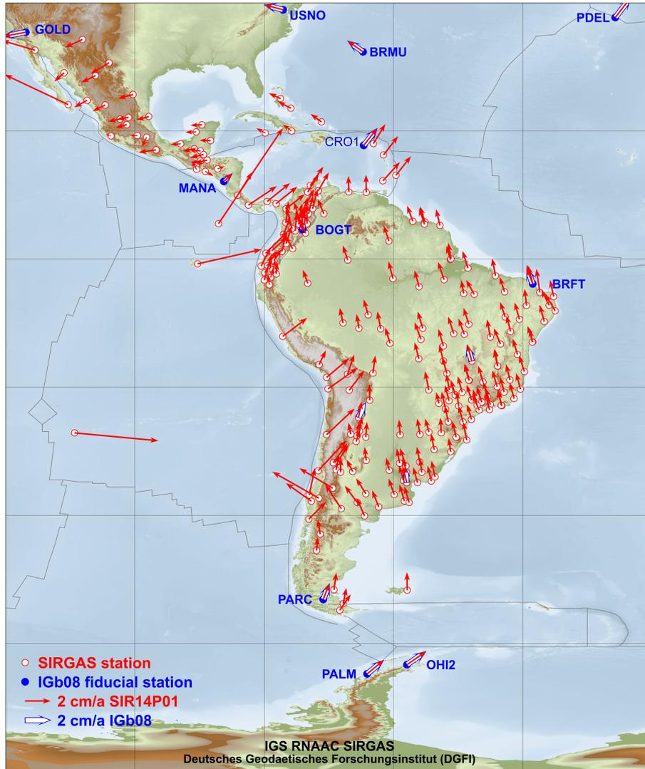
Figure 2: Horizontal velocities of the multi-year solution SIR14P01 (IGb08, 2013.0).
